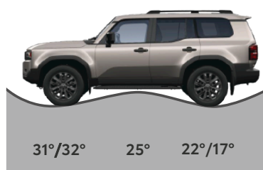
Approach, ramp break-over and departure angles (Land Cruiser / Platinum)
